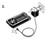
Charge the Vaporizer with a USB charger. With the optionally available USB-C Supercharger, operation is possible even if the battery is completely discharged.
